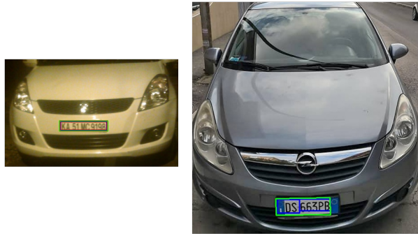
Figure 4.1: (Left) Recognition of an Indian car plate, (Right) Recognition of an Italian (European) car plate
